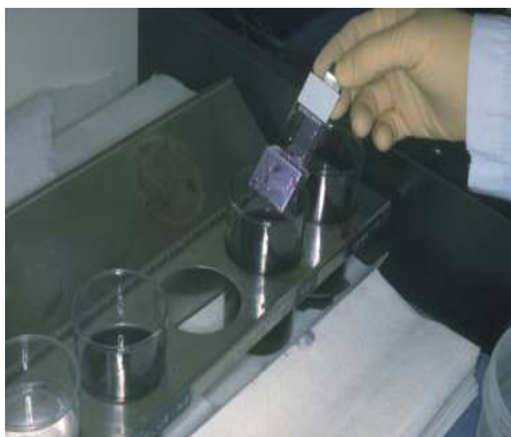
Figure 2. Process of staining slide for microscopy.
