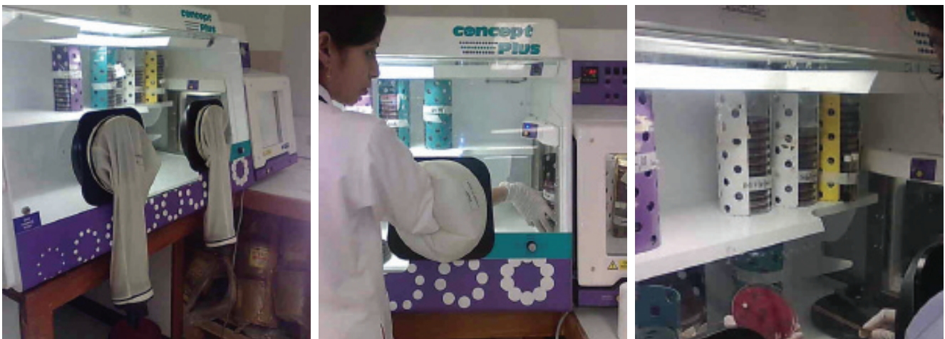
Fig 1. Anaerobic Chamber in use at Aga Khan University Clinical Microbiology Laboratory.
